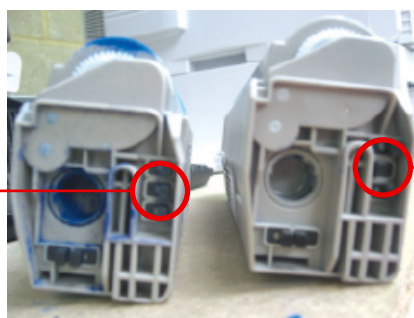
Q Imaging centre post in incorrect position (Source – OKI Printing Solutions)
