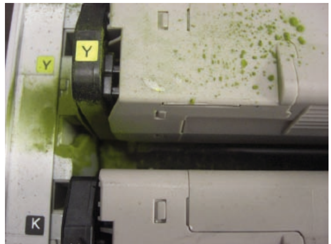
Q-Imaging Yellow imaging unit split due to toner leakage at 25,428 impressions (Source – BLI)
