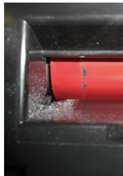
Fuser roller wear and tear at 27,639 impressions (Source – BLI)
