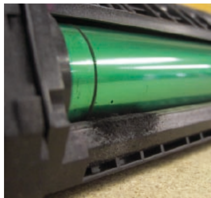
Black toner leaking in image drum causing black spots in Q-Imaging printouts at 20,413 impressions (Source – BLI)
