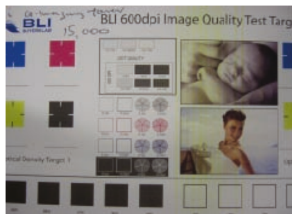
Yellow marking down centre of Q-Imaging printed output at 15,000 impressions (Source – BLI)
