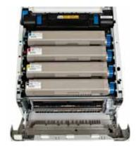
**Energy efficient, low cost printing** Power saving features such as Deep Sleep mode and auto shutdown help reduce energy consumption, whilst, high capacity, easy access toner cartridges and image drums reduce total cost of ownership and user intervention.
